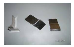
Supplied as a set of three these plain stainless steel hinges can be drilled to match the hole pattern of both the vehicle roof and the roof cap.
