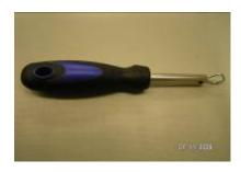
Small hand tool enables fitting of insert into main section of the window seal.
