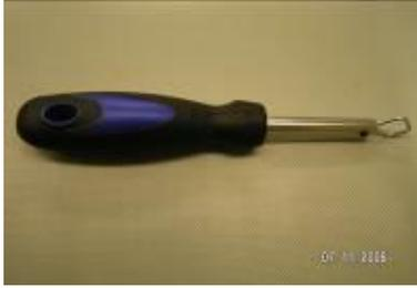
This tool enables fitting of insert/filler strip into main section of the window seal.
