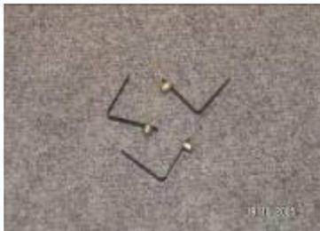
These spring pins or buttons can be used to replace the rocking strut catch normally fitted.
