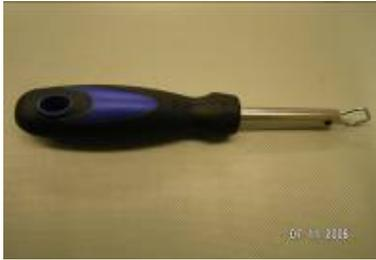
This tool enables the fitting of the insert/filler strip into main section of the window seal.
